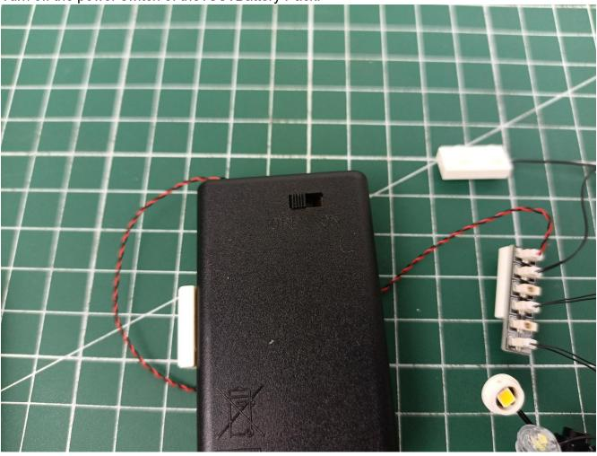
Separate AAA Battery Pack from 6-Port Expansion Boards.
