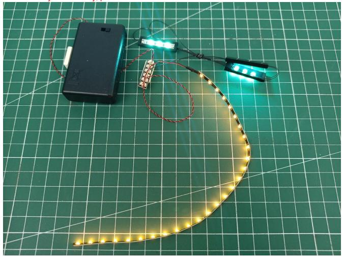
Separate the lighting from 6-Port Expansion Boards.
