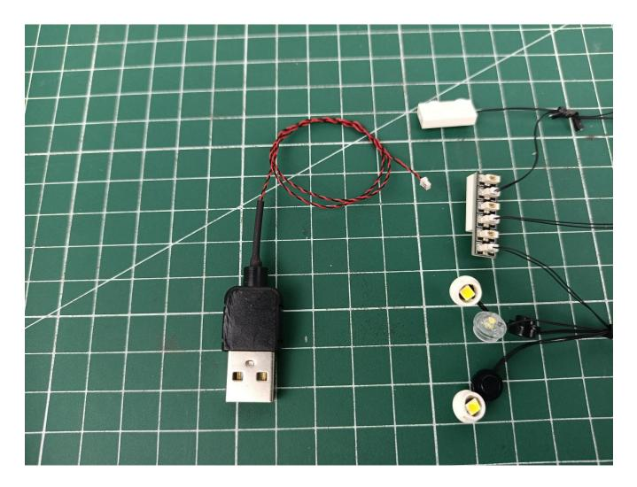
Connect the 30CM USB power cable to 6-Port Expansion Boards.
