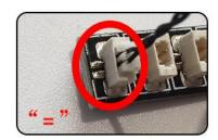
Connect the AAA Battery Pack to 6-Port Expansion Boards.
