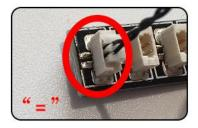
The square button battery box is equipped with batteries (batteries are self-prepared), and the power cord of the square button battery box is connected to the expansion board.
