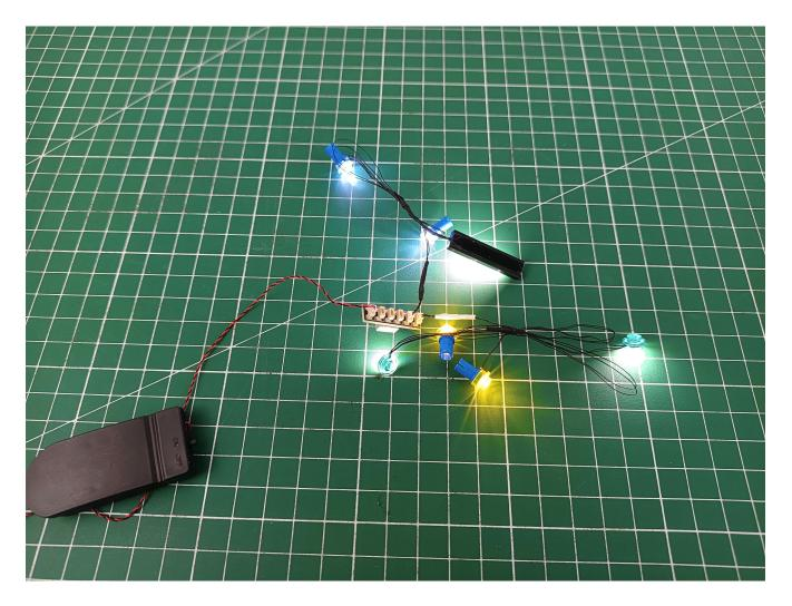
After the test is normal, unplug the lamp and be careful when unplugging the plug to avoid damaging the plug.
