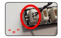
Connect the USB power cord to the expansion board, paying attention to the orientation of the terminal ports.
