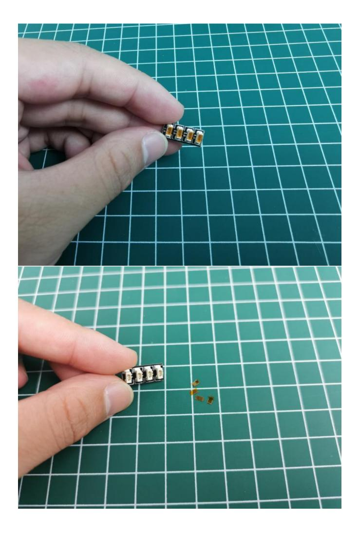
If there is a 2P interface in the package, please pay attention to the way the interface is used. The interface is small, please use it carefully: the = sign of the 2P interface is aligned with the = sign of the expansion board
