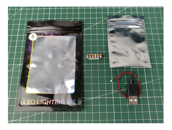
Take out 6-Port Expansion Boards and remove the protective film.
