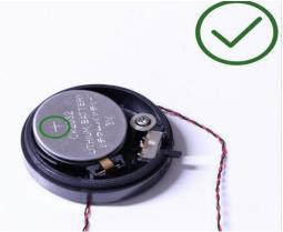
Connect Flat Battery Pack to Expansion Boards.
