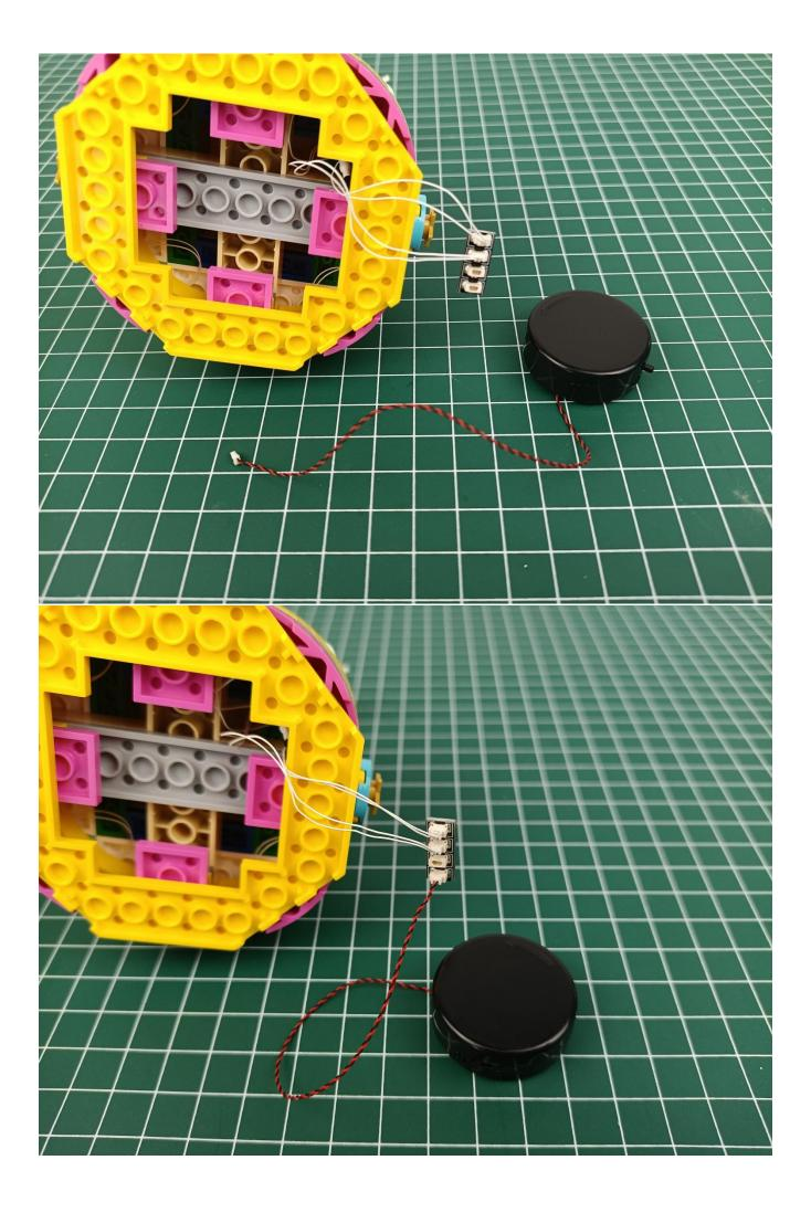
Expansion Boards are placed in the position shown in the figure, and the Flat Battery Pack is stuck in the position shown in the figure.
