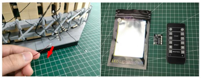
The remote control does not contain batteries, please buy a CR2025 or CR2032 button battery in the nearest store and install it in the remote control.
