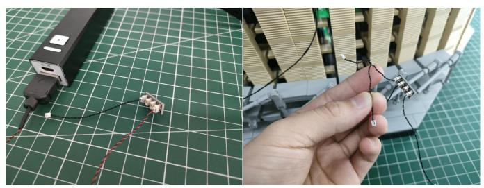
82.Connect it to the expansion board, find the connection line of the blue light, and leave it on the expansion board.
