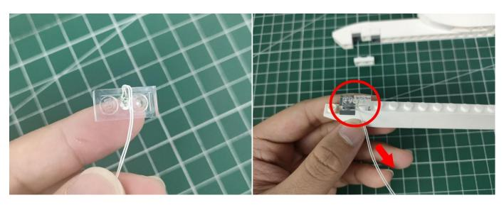
Pull the line to the right and wrap the line around the bump of the block.
