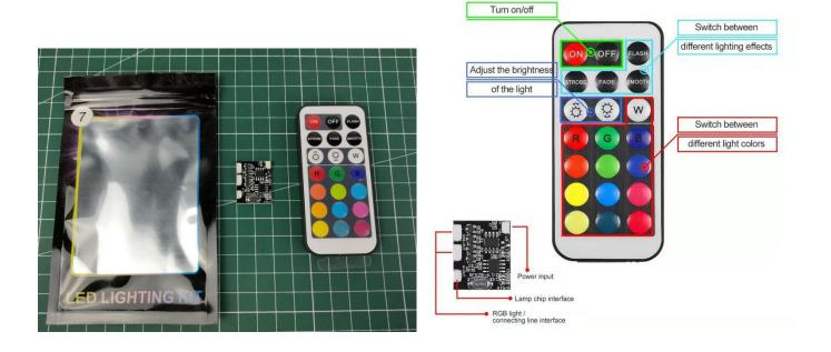
The RGB remote control does not contain batteries, please buy a 2025 or 2032 button battery in the nearest store and install it in the RGB remote control.
