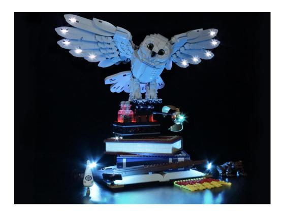
The battery box in bag NO.8 can also power the set. If it is necessary to change the power supply, prepare three AA batteries, install them in the battery box, turn on the switch on the battery box, remove the plug of the USB Power Cable from the socket of the expansion board, plug the plug of the battery box to the same socket in the expansion board to power the suit as well.
