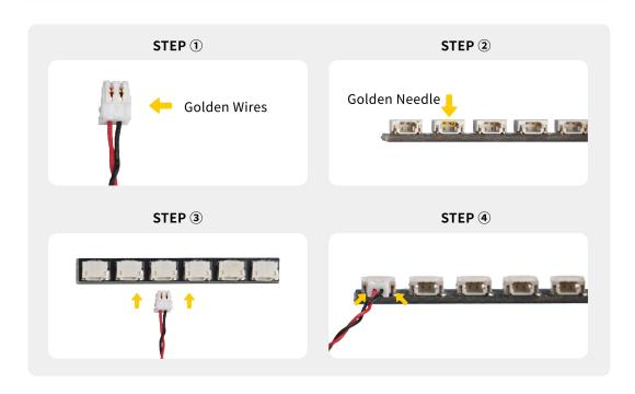
Connect the Expansion Board and USB Power Cable as shown.
