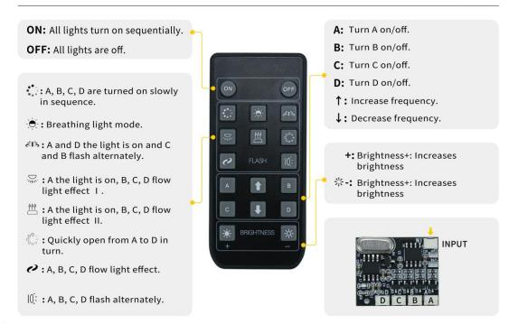
The remote control does not contain batteries, please buy a CR2025 or CR2032 button battery in the nearest store and install it in the remote control.
