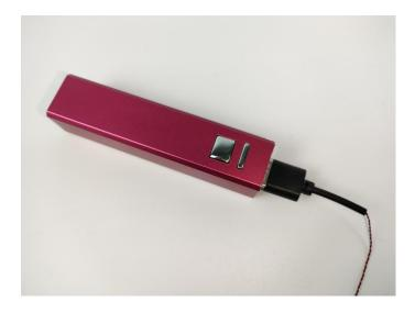
When we test "①" particles, Take out the bag labelled "①". Take out one of the light and connect it to the socket. Turn on the power bank, the light will turn on normally as shown below.
