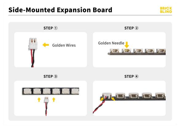
Connect the Expansion Board and USB Power Cable as shown.
