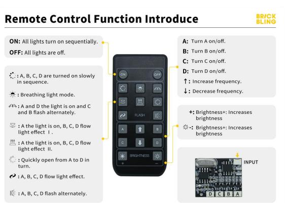
The remote control does not contain batteries, please buy a CR2025 or CR2032 button battery in the nearest store and install it in the remote control.
