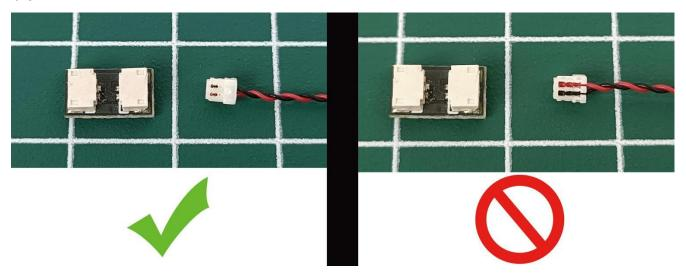
Connect the Expansion Board and USB Power Cable as shown.
