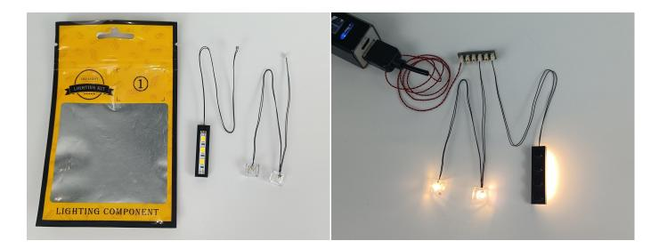
Unplug these two components and put them back in the corresponding bags. There are one in bag NO.2, four in bag NO.3, two in bag NO.4 need to be tested.
