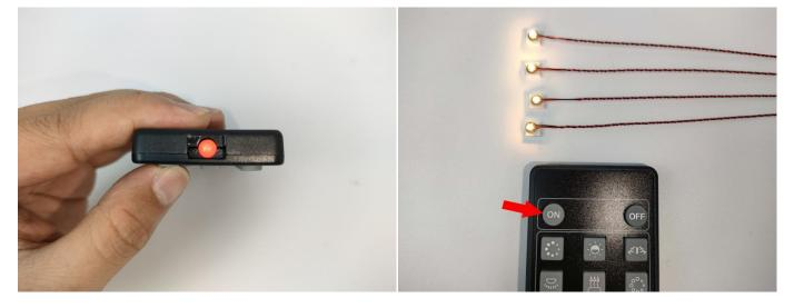
If there is any problem with the spare parts, please contact our after-sales service for replacement! Connect all the components in No.1 bag to the Expansion Board in same way just as shown.Turn on the power bank, all the lights are on as shown.Remove the lamp after the test.
