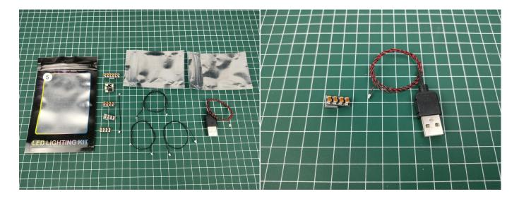
Take out the Expansion Boards and the USB Power Cable from No. 5 bag .
