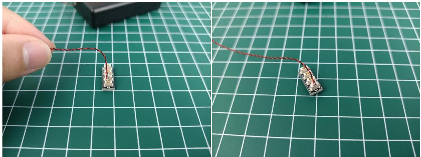
**Connect all the 2 components in No.5 bag to the Expansion Board in same way just as shown.**
