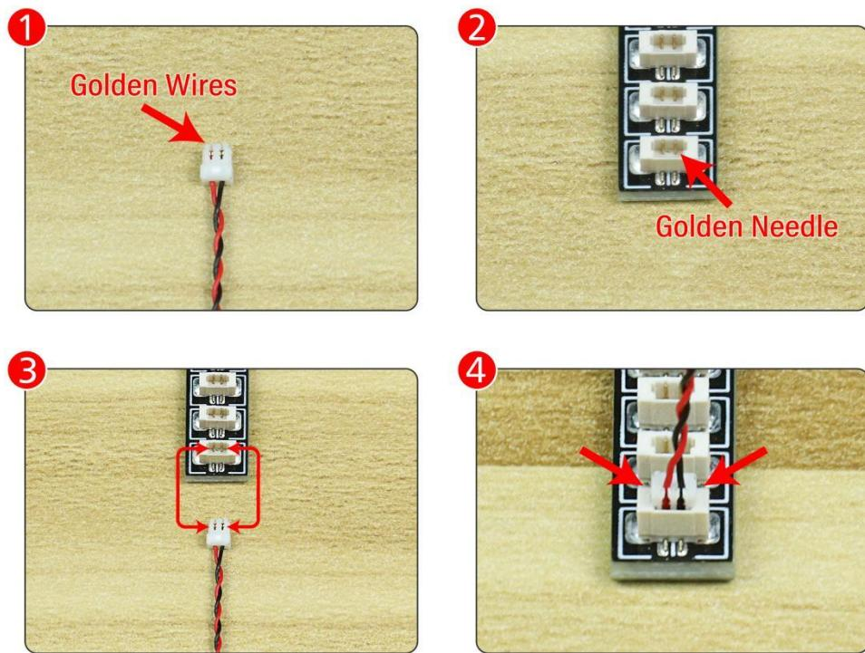
**Connect the Expansion Board and AAA Battery Box as shown.**
