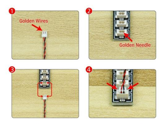
Connect the Expansion Board and USB Power Cable as shown.
