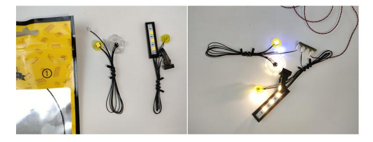
Unplug these two components and put them back in the corresponding bags. There are two in bag NO.2, two in bag NO.3, two in bag NO.4, one in bag NO.5 need to be tested. Attention that after the test is completed, each components should put back in the corresponding bag including the socket and the usb power cable.
