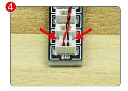
Connect the Expansion Board and AAA Battery Box as shown.
