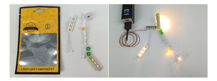
Unplug these two components and put them back in the corresponding bags. There are two in bag NO.2, one in bag NO.3 need to be tested.
