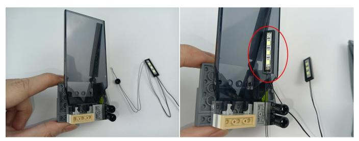
■ Push the block out of the way, then push the lamp cord through the slit in the block and push the black block back in place.
