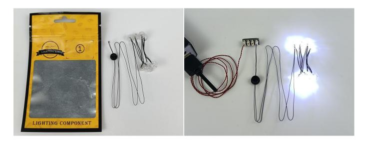
Unplug this component and return it to the appropriate bag. There are two in bag NO.2, two in bag NO.3 need to be tested.
