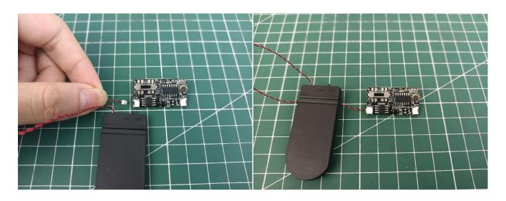
Connect all the components in No.1 bag to the Sound Control Module in same way just as shown.
