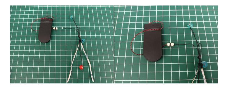
Turn on the switch on the flat battery pack, all the lights are on as shown.
