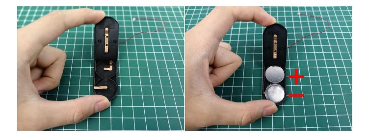
Connect the Expansion Board and flat battery pack as shown.
