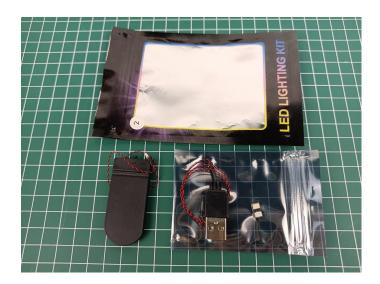
The flat battery pack does not contain batteries, please buy a 2025 or 2032 button battery in the nearest store and install it in the flat battery pack.
