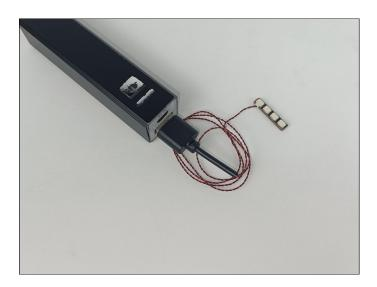
Connect all the components in No.2 bag to the Expansion Board in same way just as shown. Turn on the power bank, all the lights are on as shown. Remove the lamp after the test.
