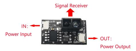
When the obstruction generate a reflected signal, the corresponding module can be turned on or off.
