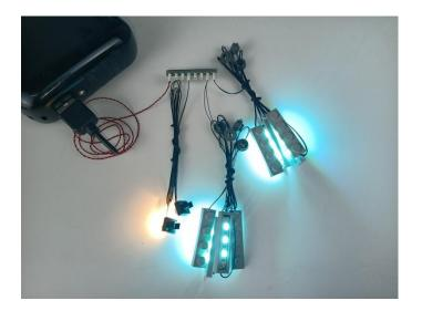
Unplug these three components and put them back in the corresponding bags. There are two in bag NO.2, two in bag NO.3,two in bag NO.4,four in bag NO.5,three in bag NO.6 need to be tested.
