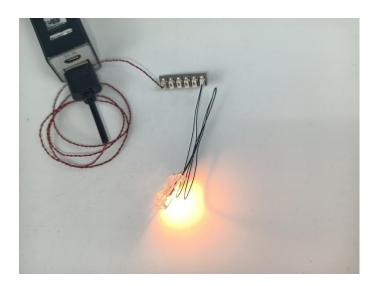
Unplug this component and return it to the appropriate bag. There are four in bag No.2 need to be tested.
