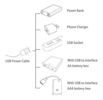
Connect the other end of the USB power cable to the power supply.
