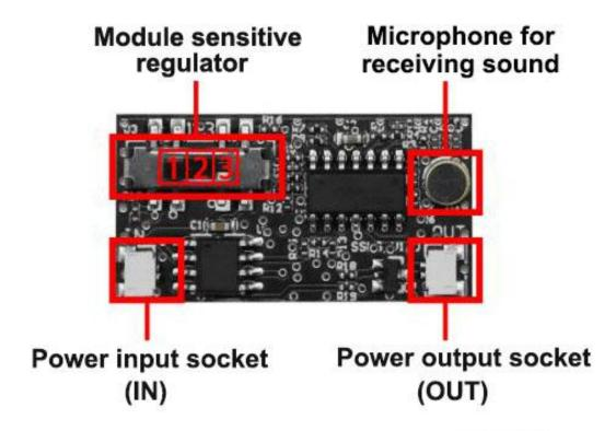
Module sensitivity adjuster. There are three gears, 1,2, and 3. The received decibels are 25dB,50dB,90dB.
