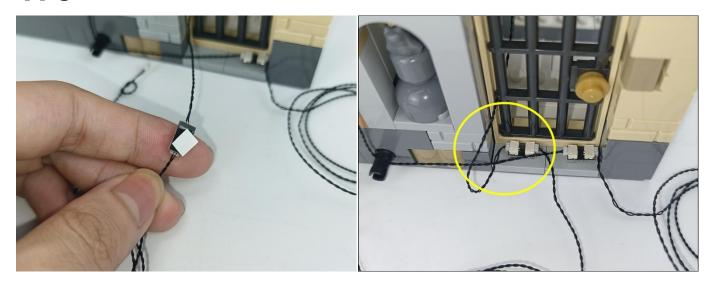
176. Pull the connecting cable on the expansion board toward the rear.
