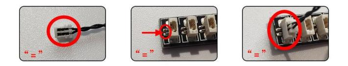
Tear off the seal on the expansion board and connect it to the port of the USB power cord.
