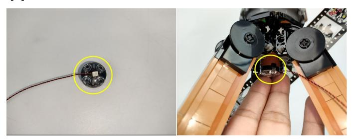
15. Place the lamp cord in the seam of the block parts, then restore the block pieces and press the lamp cord.
