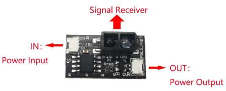
When the obstruction generate a reflected signal, the corresponding module can be turned on or off. TIPS: 1. The range of signal reception within 10cm of the vertical "signal receiver".
