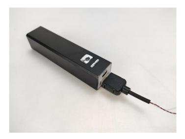
Connect all the components in No.2 bag to the Expansion Board in same way just as shown. Turn on the power bank, all the lights are on as shown. Remove the lamp after the test.
