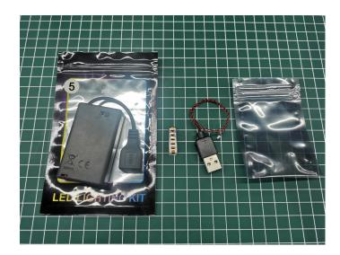
The USB AAA Battery Box does not contain batteries, please buy three AAA batteries in the nearest store and install it in the USB AAA Battery Box,connect the USB AAA Battery Box and USB Power Cable as shown.
