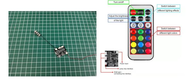
The RGB remote control does not contain batteries, please buy a CR2025 or CR2032 button battery in the nearest store and install it in the RGB remote control.
