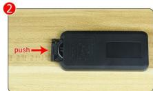
Connect the AAA Battery Box and RGB Remote Control Board as shown.
