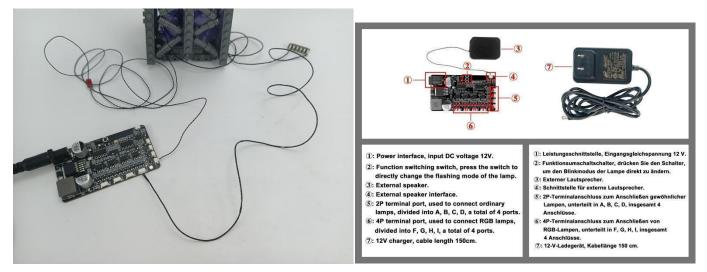
. This instruction will use the usb socket as power supply . The test structure is shown as follow. All lamp in this set will be tested by this structure.
