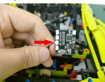
Connect the illustrated lighting line to the remote control module B port.
