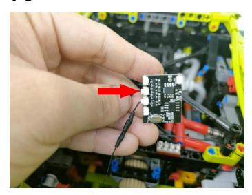
Connect the illustrated lighting line to the remote control module D port.
