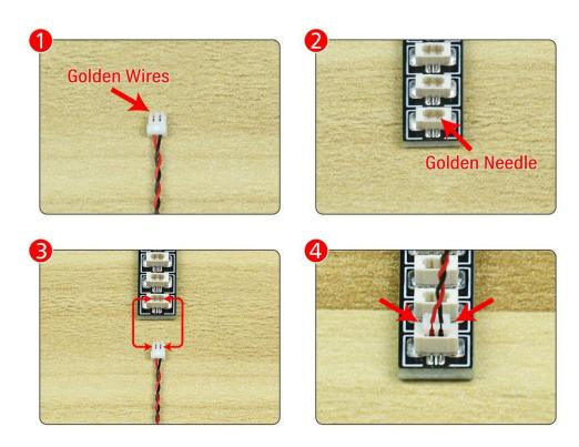
Connect all the components in No.1 bag to the Expansion Board in same way just as shown.
