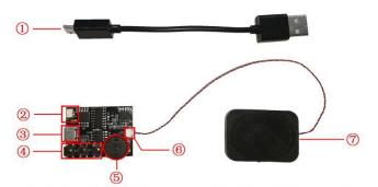
①:USB data cable is used to connect modules to the computer to replace music files.
