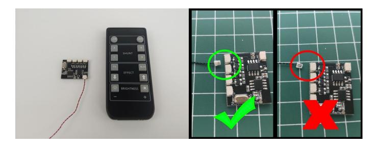
Connect one components in No.1 bag to the Remote Control in same way just as shown.
