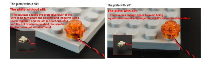
The slit on the plate round 1X1 are hand-made to avoid squeeze the wire and cause short circuit and abnormalheat during installation.
