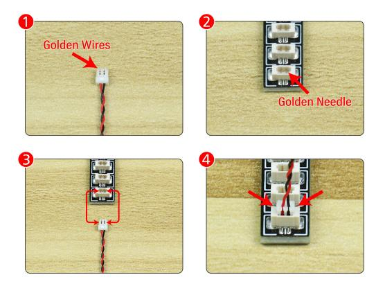
Connect the Expansion Board and USB Power Cable as shown.
