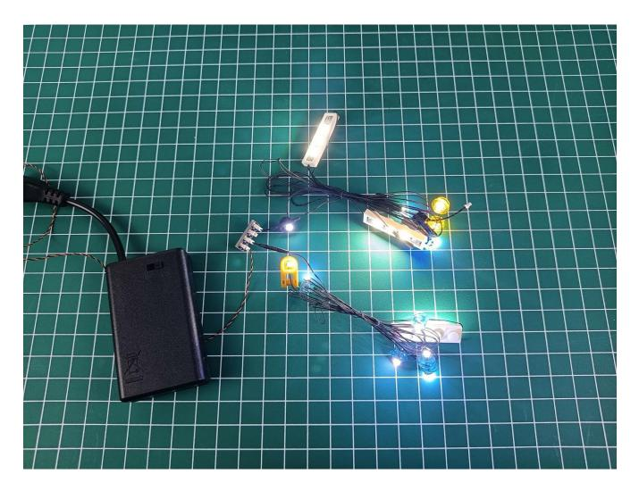
If there is no abnormality, unplug the lights and leave the expansion board on the USB power cord, Put the lighting back into the original bag, and test the lighting of other bags in the same way.
