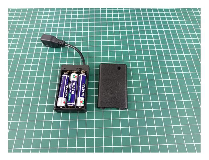
Connect the USB power cord to the battery box.
