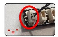
Tear off the seal on the expansion board and connect it to the port of the USB power cord.
