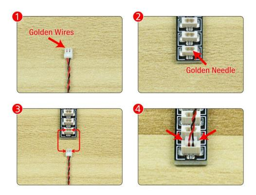
Connect the Expansion Board and AA Battery Box as shown.
