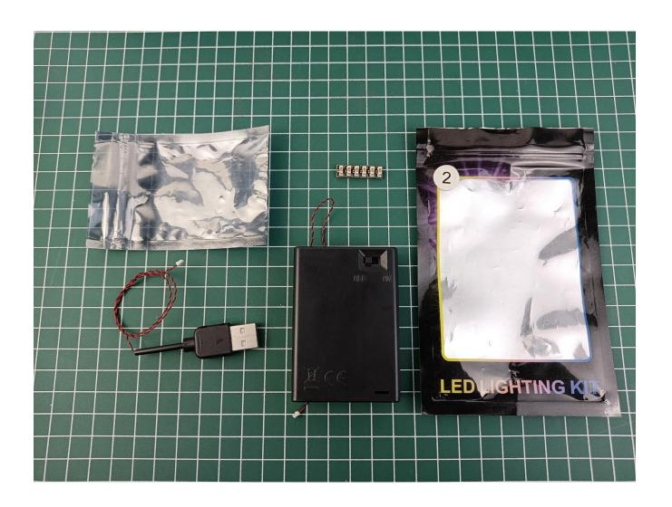
Take out the USB power cord and a 6-Port Expansion Boards, and then tear off the seal of the expansion board. Coming with usb cable and battery box for choose, can be powered by power bank/wall charger or you can also use it with the battery.
