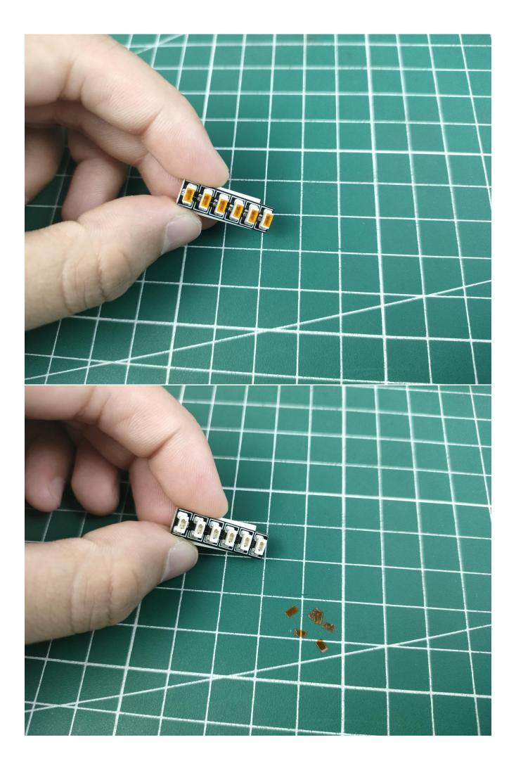
Please pay more attention and carefully using the connector for it is small.The "="of the 2P interface is aligned with the "=" of the expansion board.The "=" on the expansion board refers to the two outside solder joints, not the two metal pins inside the jack.
