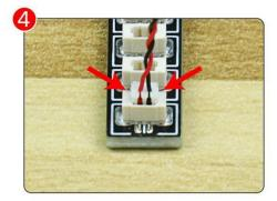
Remove the protective film from the Expansion Boards. Connect the Expansion Board and USB Power Cable as shown.
