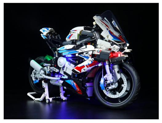
The battery box in bag NO.4 can also power the set. If it is necessary to change the power supply method, prepare three AAA batteries, install them in the battery box, turn on the switch on the battery box, remove the plug of the USB Power Cable from the socket of the expansion board, plug the plug of the battery box to the same socket in the expansion board to power the suit as well.
