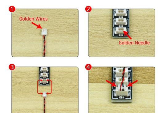
Remove the protective film from the Expansion Boards. Connect the Expansion Board and USB Power Cable as shown.
