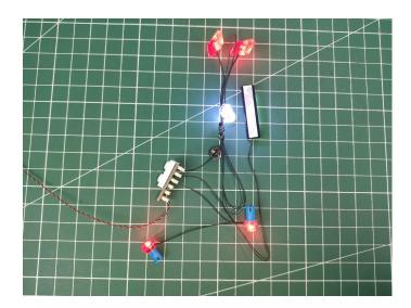
Unplug these three components and put them back in the corresponding bags. There are three in bag NO.1, two in bag NO.3 need to be tested.
