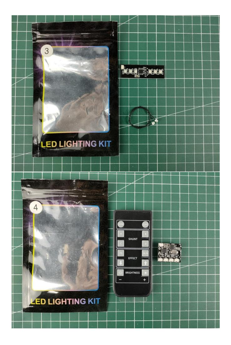
Take out the USB power cord, remote control, and remote control module. The usage of the USB power cord is similar to that of the battery box, and it can be powered by a power bank or a mobile phone charger. The battery box and the USB power cord can be freely chosen, choose one of the two (the USB power cord used in this article).
